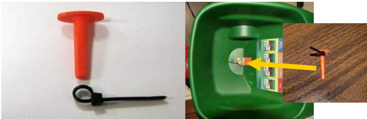
Cable tie ready for placement (left) with agitator re-attached (right)
