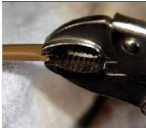
Squeeze the tip almost closed with a pair of pliers or vice grips.
