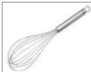
A kitchen whisk can be modified to fit into the drill chuck.
