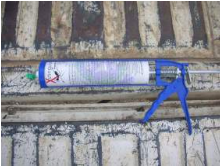
Figure 6. A tube of Xstinguish™ housed in a caulking run and ready for use. The small amount of bait (coloured green) next to the nozzle is approximately the correct amount to apply in each spot.
