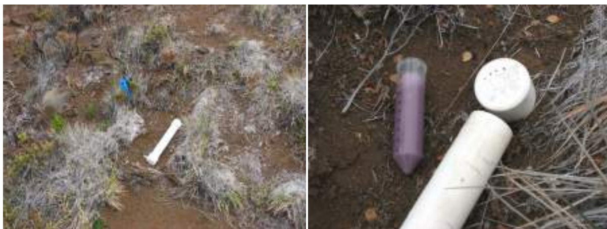
Figure 1. Bait station design chosen for the experimental plots. The panel on the left shows placement of a bait station in the field, while the panel on the right shows a close-up view of one endcap (removed) with the four entrance holes, as well as an internal bait tube containing bait stoppered with a cotton ball.
