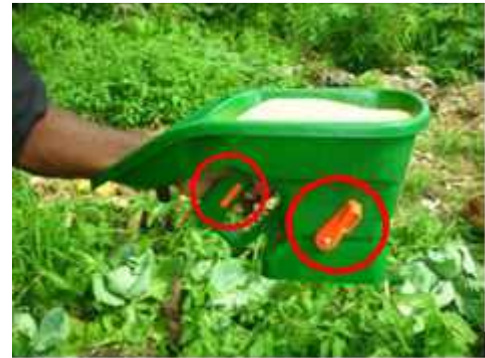
Typical hand held bait spreader showing the winding handle and the aperture adjustment. Set the aperture at “1”.
