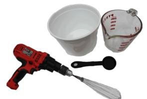
A device for mixing. We use a cordless drill with a kitchen whisk modified so it can be fitted into the drill chuck. A paint mixer also works well in place of the whisk.
