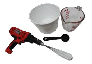
A device for mixing. We use a cordless drill with a kitchen whisk modified so it can be fitted into the drill chuck. A paint mixer also works well in place of the whisk.
