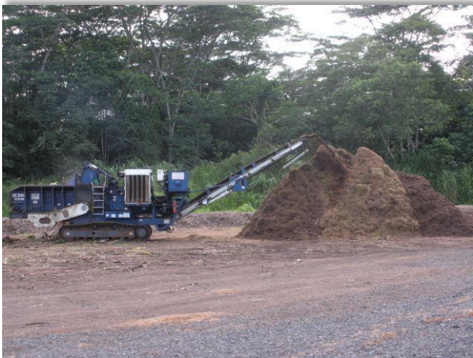
Hilo green waste mulching machine in action
