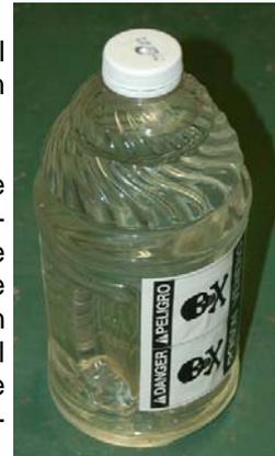
Figure 6. Prepared bottle. Note pesticide labels, and the hole drilled in the bottle cap.
